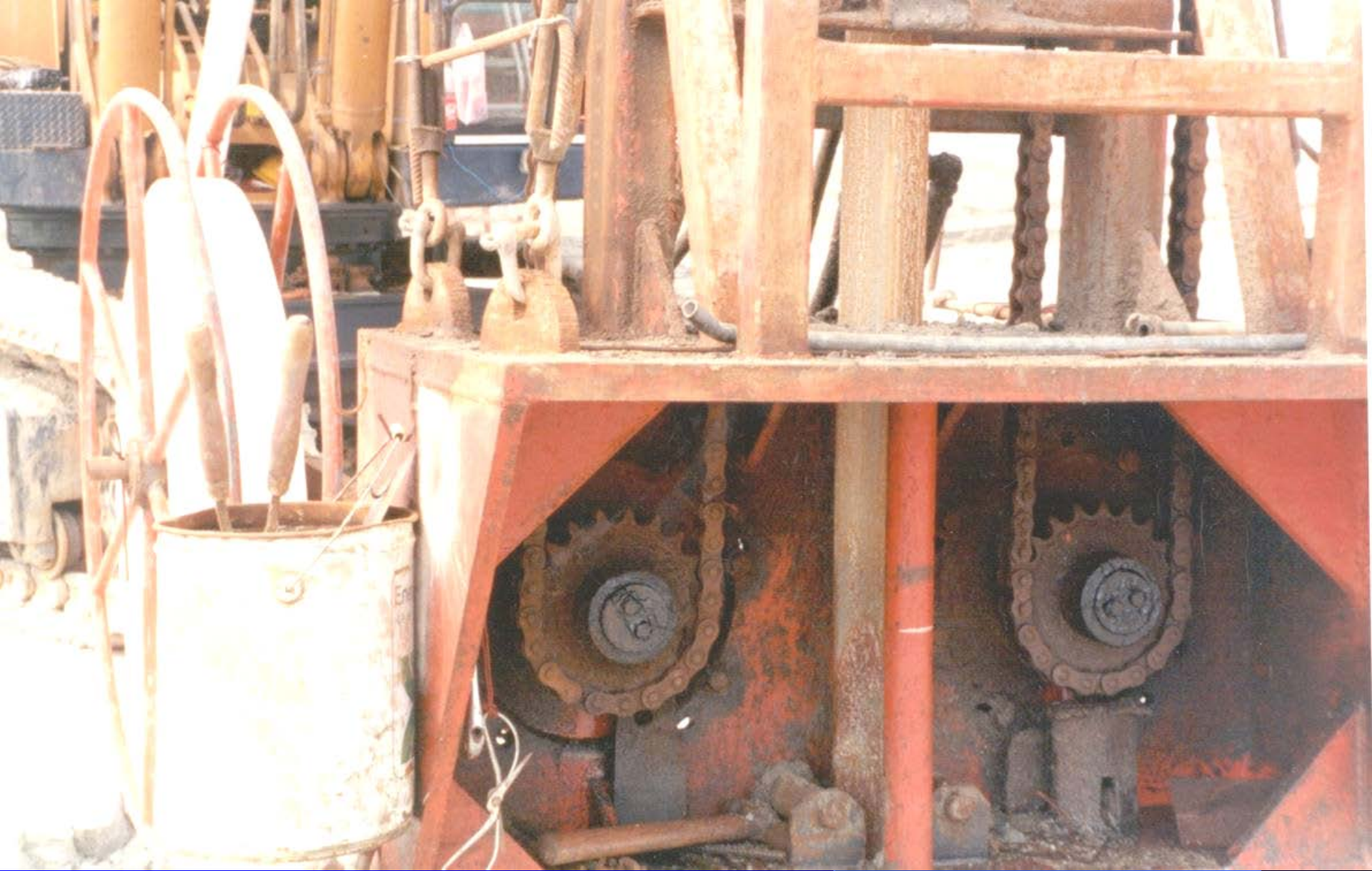
Close up chain drive system
