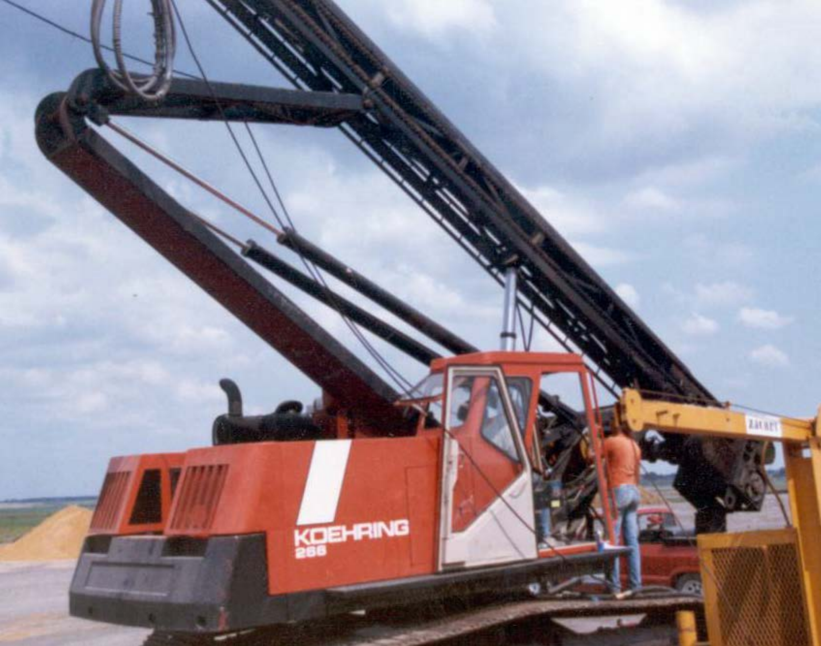
Self erecting static/top drive vibro with chain drive.
