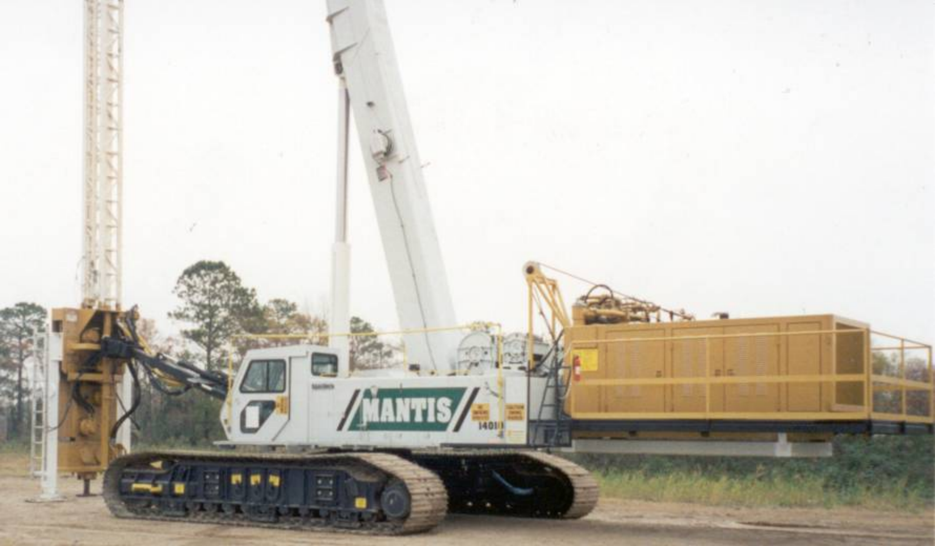
APE Bottom drive wick machine mounted on a Mantis 70 ton crane. Higgerson Buchanan Inc. Chesapeake, VA
